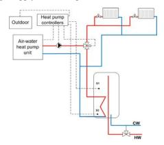
Figure 1: Schematic diagram of directly coupled (reference) heating system configuration
