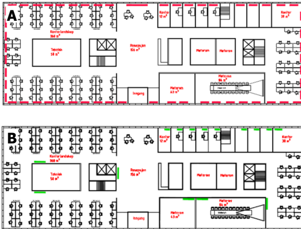
Figure 24 Example – traditional design (A) and simplified design (B) for a radiator system for space heating in a 3200 m 2 office building of passive house standard (Smedegård et al., 2012).
