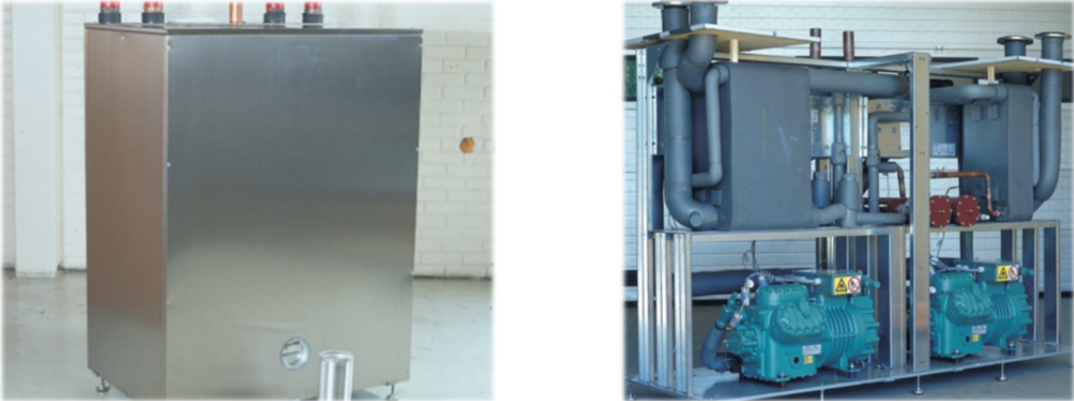
Figure 23 Low-capacity single-stage propane heat pump/chiller units with DX evaporators and reciprocating compressors (2013). Maximum outlet water temperature 50-55 °C.
