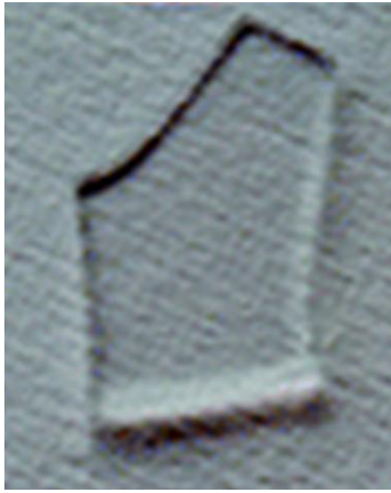
Figure 1 Photo (left) of a new developed glass material with reduced mass density (weight), reduced thermal conductivity and increased solar transmittance (right).
