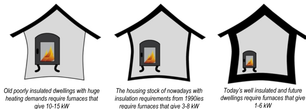
Figure 1 Picture illustrating the reduced power needs of the house with increased insulation level (from StableWood project).
